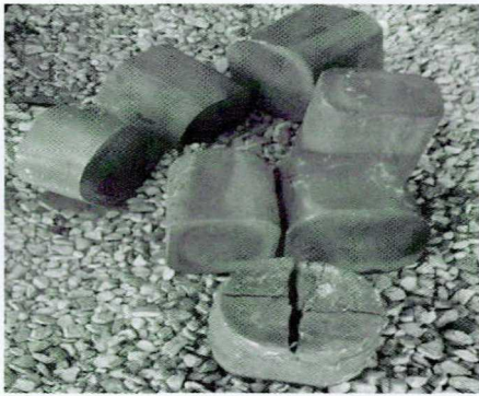
图 2 S32707 (AG-2) 钢 200 mm × 140 mm 锻坯开裂照片 Fig. 2 Photograph of steel S32707 (AG-2) 200 mm × 140 mm cracking forged billet
